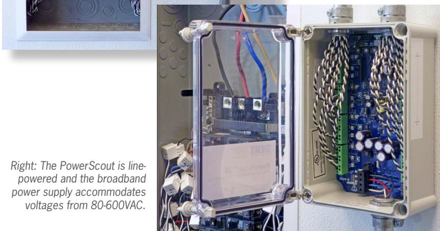
Right: The PowerScout is line-powered and the broadband power supply accommodates voltages from 80-600VAC.
