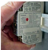
DIN-rail mount is standard
